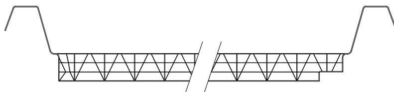
The **Easyroof®** and **Easypanel** panels are multiwall polycarbonate panels designed for use in the construction industry. They are mainly used for flat roofs in combination with sandwich panels or corrugated metal profiles.
